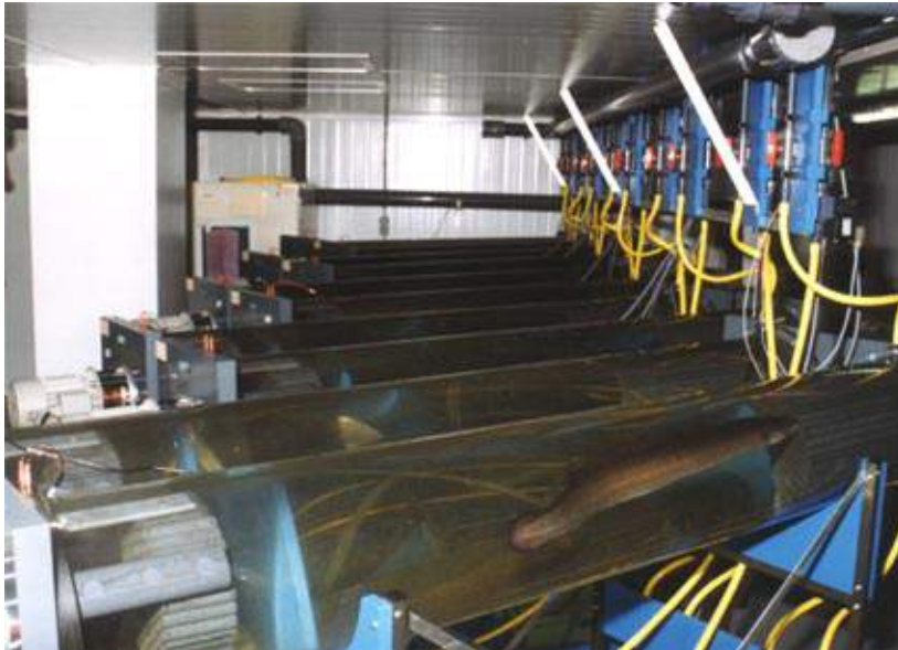
2m length A) motor; B) propeller; C) external tube; D) internal tube; E, honey comb; F) swimming section (1m); G) honey comb
